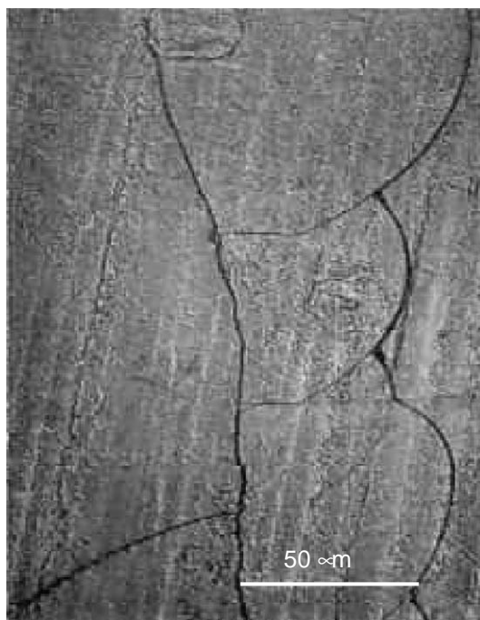
Fig. 5. Typical optical micrograph of Ar plasma-treated PDMS showing curvy cracks.
