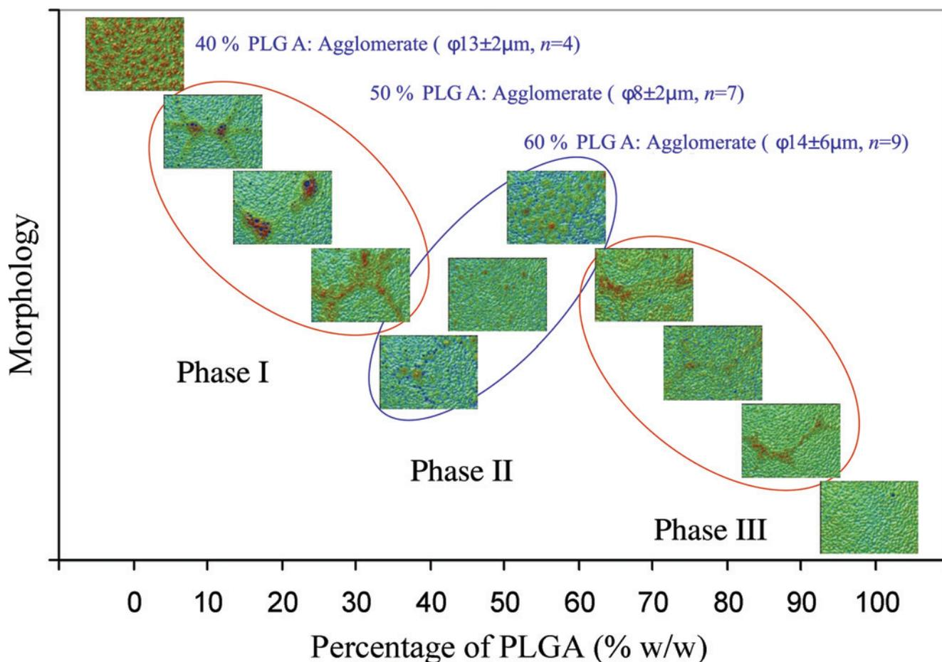
Figure 1. Morphologies of entities of PLGA or PCL frozen in PCL or PLGA ( $92 \mu\text{m} \times 121 \mu\text{m}$ ). This figure is available in colour online via [www.i-cheme.org/cherd](http://www.i-cheme.org/cherd)
